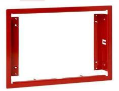
The Avenger trim ring allows the eVIEW annunciator to easily be recess mounted. Avenger trim rings provides placement tabs that fold behind dry wall. Traditional screw mounting is available by 2 openings in each of the vertical frames. Conduit entry is not blocked by trim ring.
