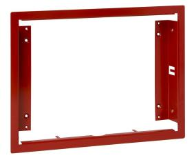
The VES trim ring allows the eVIEW annunciator to be easily recess mounted. Avenger trim rings provides placement tabs that fold behind dry wall. Traditional screw mounting is available by 2 openings in each of the vertical frames. Conduit entry is not blocked by trim ring.
